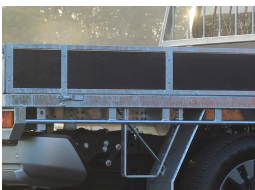
Steps and tie rails
