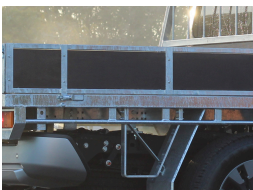
Steps and tie rails
